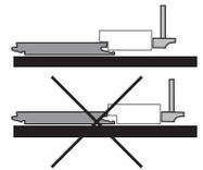
**the planks** (e.g. when installing final row) tap planks together gradually. Begin tapping lightly at the corner of a plank until the joint has clicked together. Repeat the process approximately every 12" (30cm) until the entire long edge of the plank has clicked in with the next plank.
