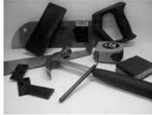
When sawing pieces off the planks, use a fine-toothed hand saw, jigsaw, chopsaw, guillotine or utility knife.
