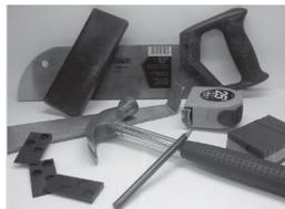
When sawing pieces off the planks, use a fine-toothed hand saw, jigsaw, chop-saw or guillotine.
