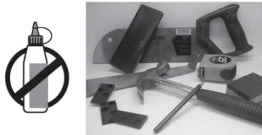
When sawing pieces off the planks, use a fine-toothed hand saw, jigsaw, chop-saw, guillotine or utility knife.
