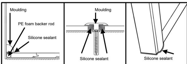
\*For **non-waterproof** installations, PE foam backer rod and silicone sealant are not required.
