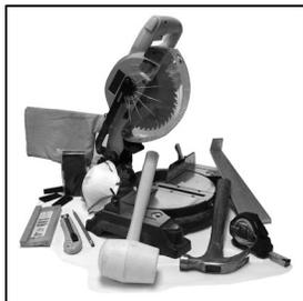
When sawing pieces off the planks, use a fine-toothed hand saw, jigsaw, chop-saw or guillotine.
